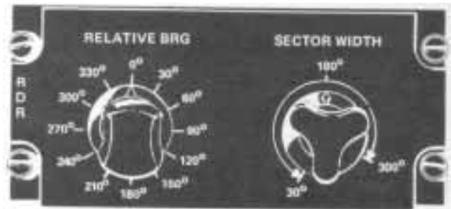
ANTENNA CONTROL PANEL
