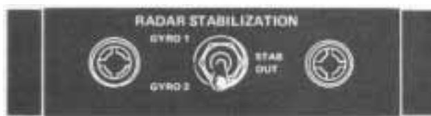
RADAR STABILIZATION CONTROL PANEL
