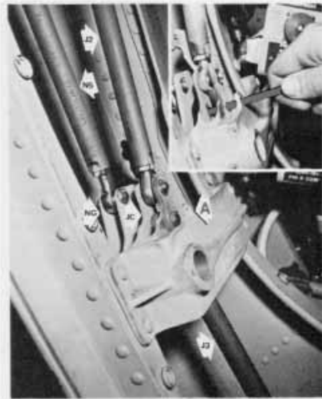
Figure 8. A rig pin installed in the rigging hole (A) will keep the outside handle in a fixed position while adjustments are being made (see inset).
