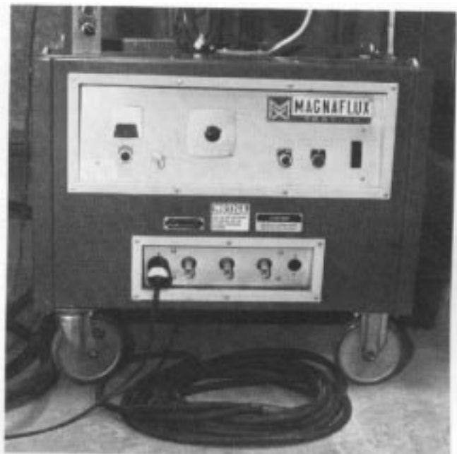
Figure 3. M-500 mobile power pack used in magnetic particle evaluation.
