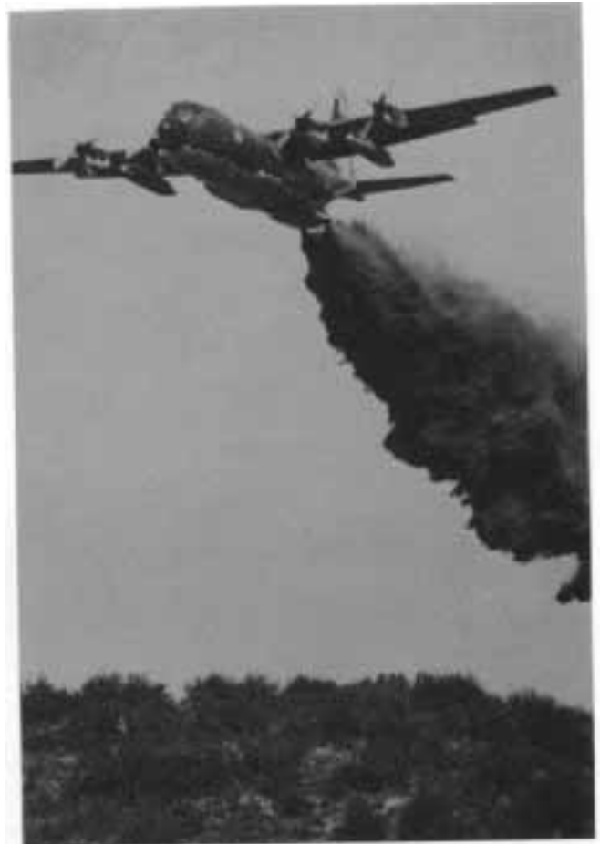
The chemical retardants used to attack forest fires can attack airframes as well.
