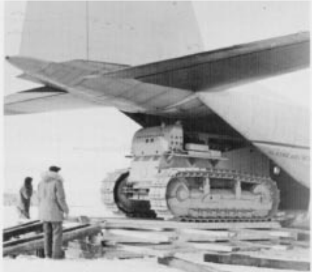
Plywood shoring can protect the cargo floor from damage caused by heavy equipment.
