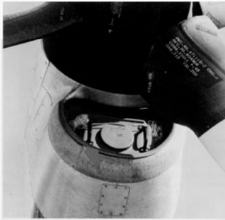
The regular use of covers will help keep snow and ice out of intakes, ports, and other openings.
