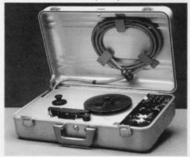
Figure 5. With this ground support tape unit, the 25 hours of recorded DFDR data can be copied in just 16 minutes.
