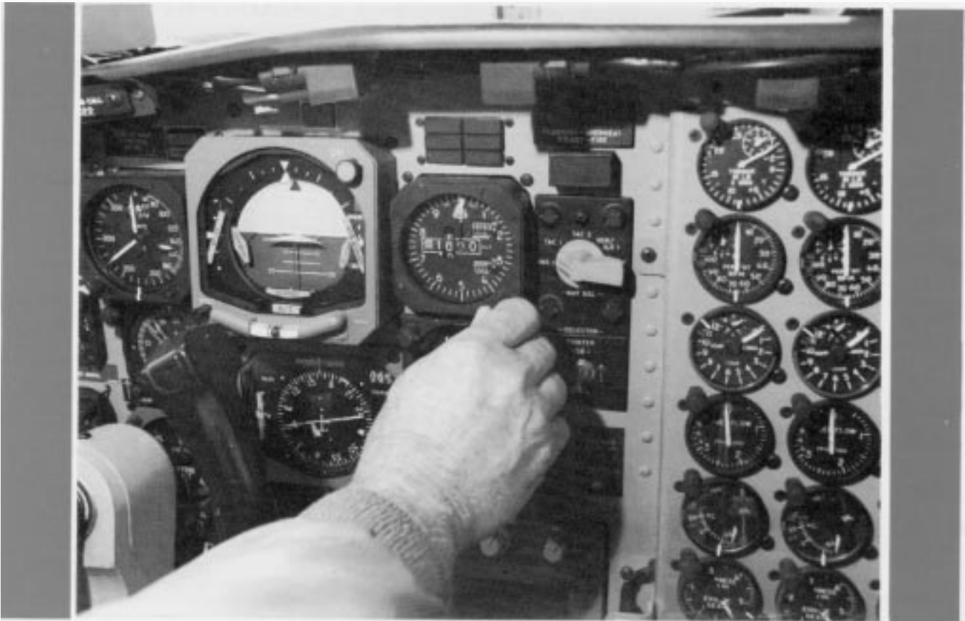
Figure 4. Pressure altitude is also a critical parameter. Averaging the readings obtained from two flight station altimeters reduces the chances of error.
