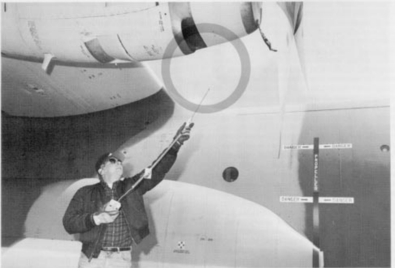
Figure 3. The ambient air temperature must be measured as accurately as possible for valid engine performance results. Be sure to take temperature readings in a shaded area.
