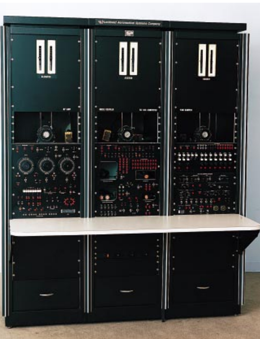
The AP-105/FD-109 Integrated System Test Set: C-130 field level.
