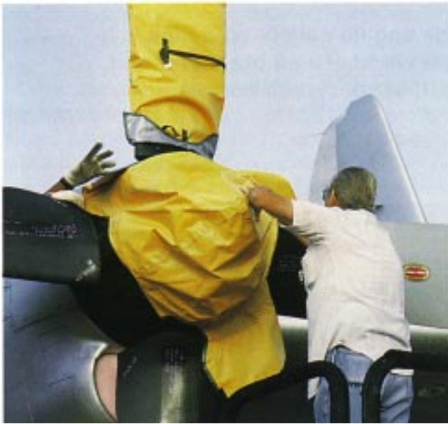
The large spinner cover fully protects the entire spinner.
