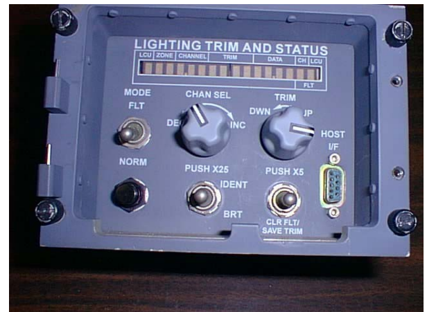
Trim and Status Panel (STP)
