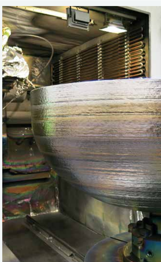
3-D printing products, like this satellite fuel tank, can reduce production time, ensure product specifications and help mitigate the risk of counterfeit parts in the supply chain.
