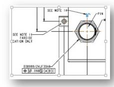
Example: MIL-DTL-38999 has the requirements for the hole size for the connector illustrated as well as torque requirements.
