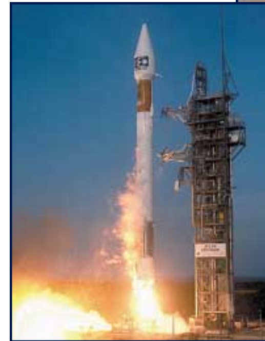
The Atlas III launcher, powered by the Russian RD-180 engine, successfully launched for the first time last year. Atlas III represents the fifth consecutive Atlas model—all of which launched successfully on their first missions. Between 1993 and 2000 Atlas launchers have flown a total of 54 consecutive successful missions.
