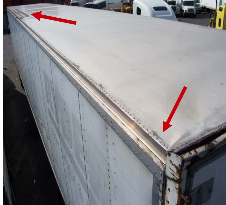
New Rivets / Repairs
